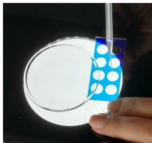
Figure 3. 5: Microscope slide with eight cavities used to individualize larvae to classify mobility following the scale presented on the right.
