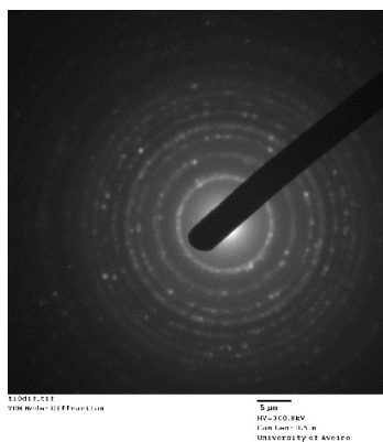
Fig. 17 – Diffraction pattern of nTiO 2 (polycrystal)
