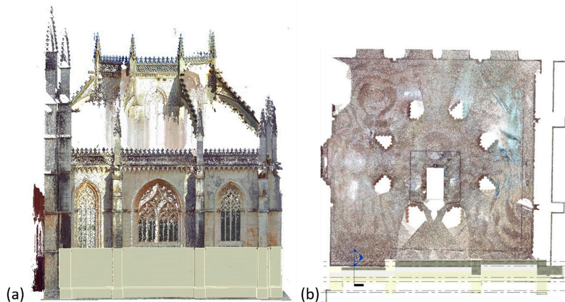
Figure 13. (a) Three-dimensional view of the wall object of the façade, (b) plan view of the point clouds superposed to this wall object.
