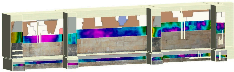
Figure 15. Images and maps on the bottom part of the chapel façade integrated in the BIM model.
