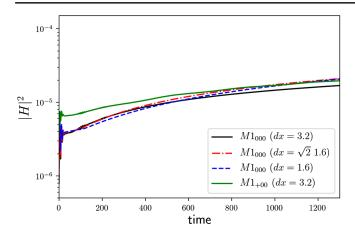
FIG. 6. Convergence for run  $M1_{000}$ : Evolution of the L2-norm of the Hamiltonian constraint for three different resolutions rescaled to show fourth order convergence. Green line shows L2-norm of the Hamiltonian constrain for a perturbed run, initially, the violation of the constraint due to the perturbation is evident, as time passes the magnitude of the error is comparable with the error of the unperturbed runs.
