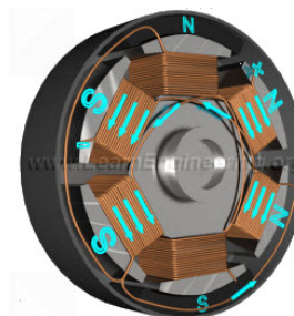
(g) Connected winding produces exactly same current flow as that of the separately energized state.
