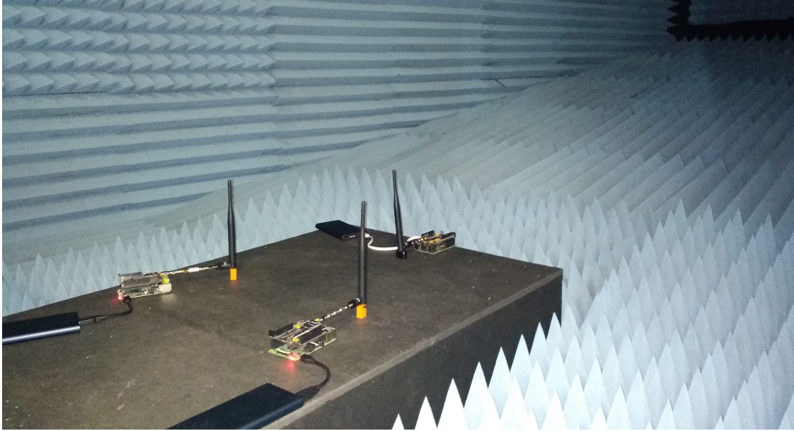
Figure 3.3: Experimentation setup with one gateway and two end-nodes.
