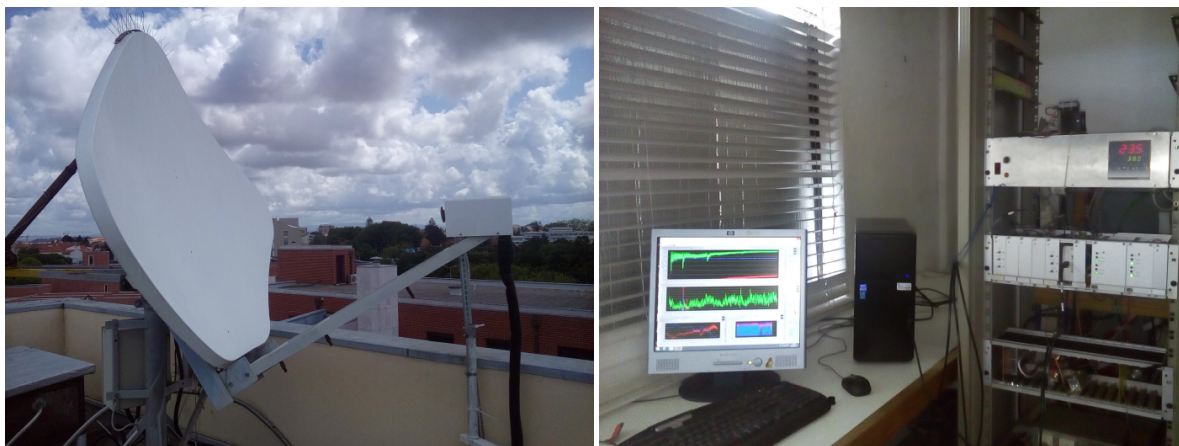
(a) Receiving antenna and front-end at DETI: Ka-band. (b) Ka-band receiver indoor part: hardware and acquisition PC.
