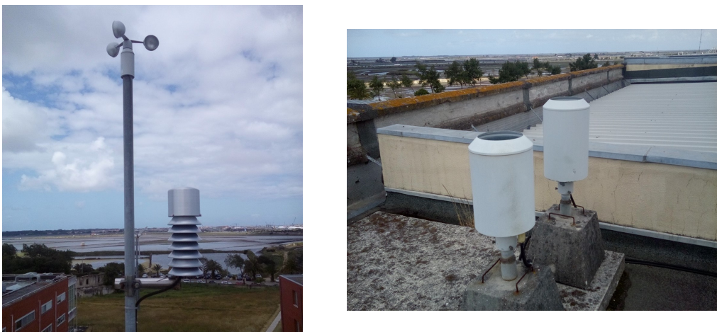
Figure 5.3: Wind speed and wind shield containing temperature and humidity sensors (left); the two rain gauges (right).
