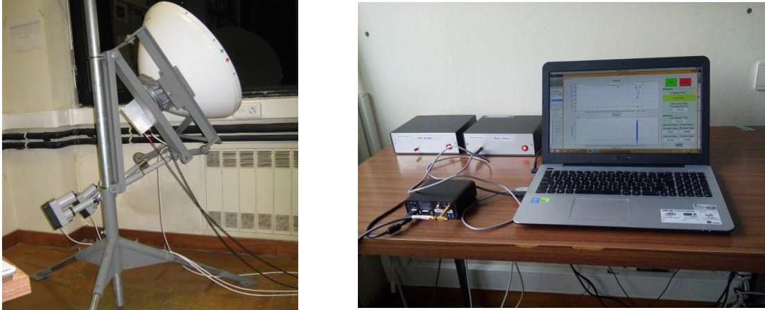
Figure 5.2: An aspect of the Q-band beacon receiver: the antenna, down converters and antenna pointing actuators (left) and SDR, antenna controller, reference frequency source and data acquisition (right).
