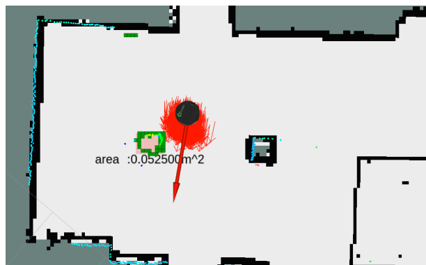
Figure 4.13: Occupied area 2. The green blocks delimit the occupied area and the calculated area is displayed.
