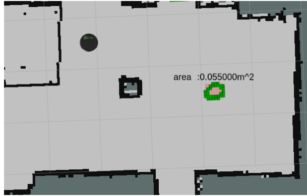
Figure 4.5: Occupied areas. The black dots and the light grey areas represent the map already created. The green blocks delimit the occupied area and the calculated area is displayed.
