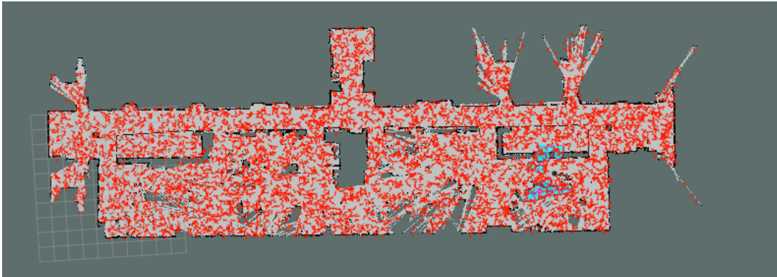
Figure 2.8: AMCL starting algorithm, with the red arrows representing possible positions of the robot scattered on the map
