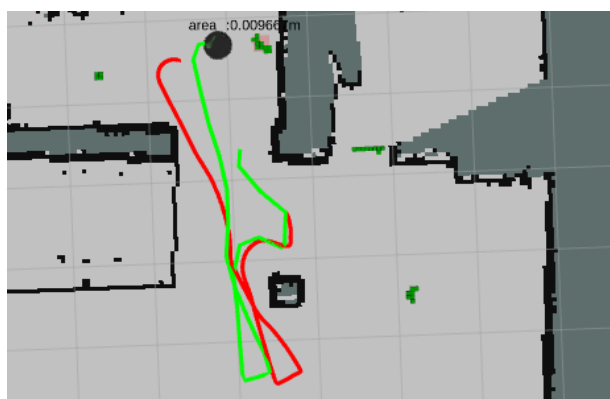
Figure 4.18: Location by odometry (red) compared to AMCL (green) for small distances, with initial position error
