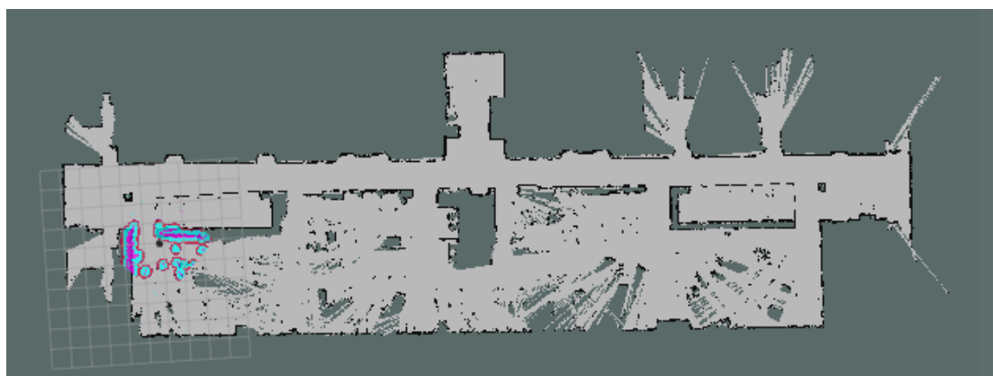
Figure 2.7: Map generated by GMapping in the ROS environment using this robot on the 1st floor of the IEETA
