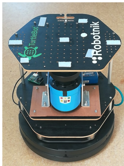
Figure 3.3: Turtlebot, used in this dissertation with the LiDAR at the front
