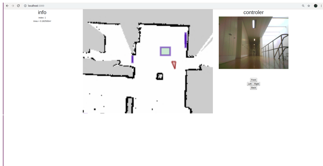
Figure 4.17: Web page of the map of the third test. The blue squares represent the occupied areas.
