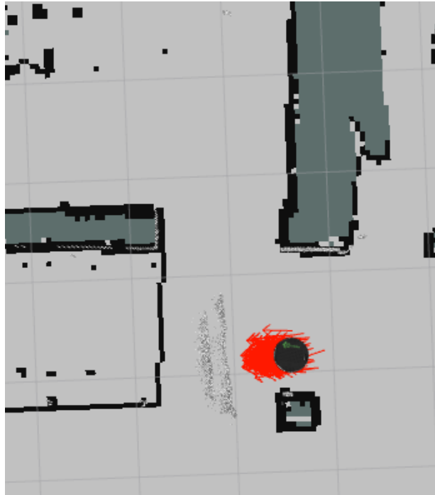
Figure 4.4: The black dots and the light grey areas represent the map already created. The white dots is a stack of some readings of the LiDAR and the black circle the most probable position of the robot.
