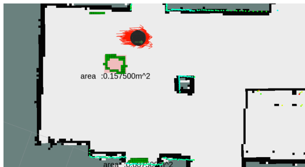
Figure 4.10: Occupied area 1. The green blocks delimit the occupied area and the calculated area is displayed.
