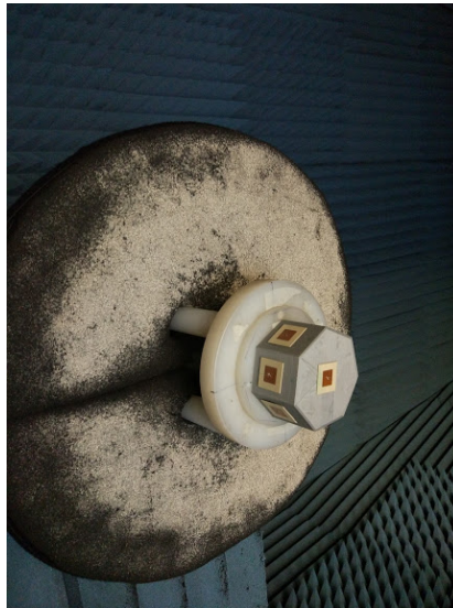
Figure 4.18: Antenna array measurement in anechoic chamber.
