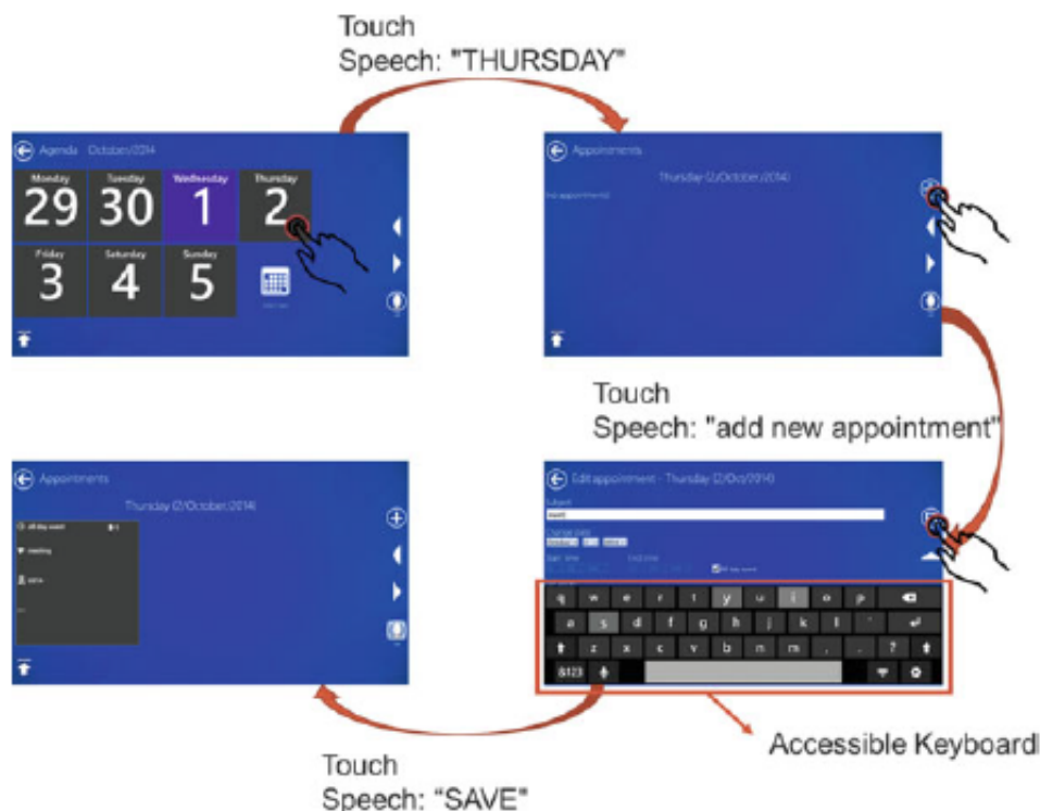
Figure 2.30: “Interactions flow to create a new appointment in the agenda, the user starts by choosing the preferred way to interact with the application (touch or speech) to select the day and then select the option to add a new appointment, then fill the subject with the virtual keyboard, and again select to save the appointment by touch or speech” (Teixeira, S. Silva, et al., 2016).
