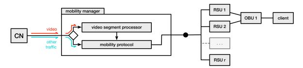
FIGURE 3.5. Position of this work's proposed solution main component, in the VANET topology. The main component, named "video segment processor," reacts to the video stream packets that enter the mobility manager, giving hints to the mobility protocol on which RSU path to choose.
