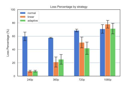
FIGURE 5.10. Loss Percentage on all video resolutions by strategy in static tests.
