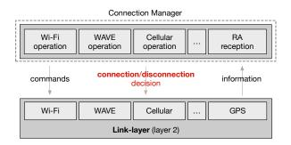
FIGURE 2.15. Detail of Connection Manager components and interaction with OSI's link-layer (layer 2).
