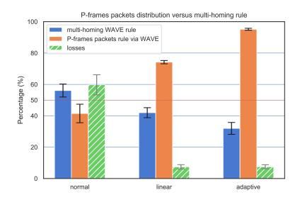
FIGURE 5.3. P-frame packets distribution in comparison with applied multi-homing rule in static 240p experiments. The losses in the plot are a copy of those in figure 5.2.
