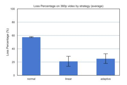
FIGURE 5.4. Loss Percentage on 360p video resolution by strategy in static tests.
