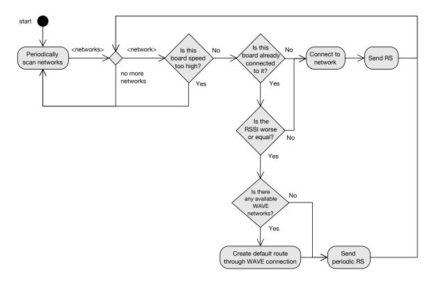
FIGURE 2.18. Wi-Fi networks processing thread in Connection Manager.
