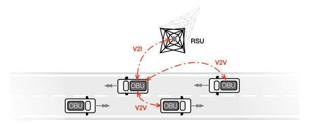
FIGURE 2.1. Common topology of a VANET and V2I and V2V communications. The RSUs form an infrastructure which provides network service to other nodes positioned on vehicles. These nodes can establish V2I and V2V communications.
