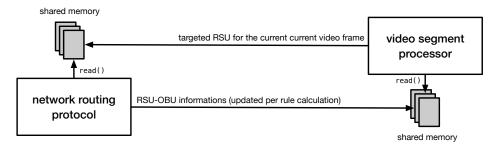
FIGURE 4.2. Message exchanges between the video segment processor and the network routing protocol.
