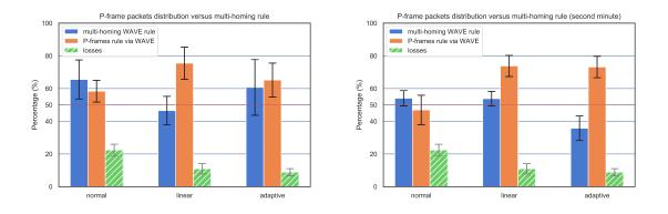
FIGURE 5.19. P-frame packets distribution in comparison with applied multi-homing rule in outside 360p experiments. The losses in the plots are a copy of those in figure 5.18. More, the plot on the left shows the results of the complete experiments, and the plot on the right shows the results in the second minute of all five experiments.
