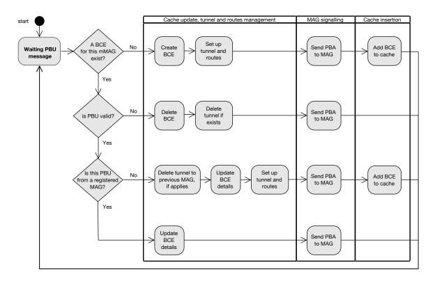
FIGURE 2.10. The LMA operation finite state machine.
