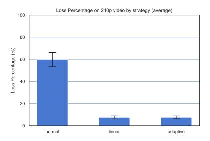
FIGURE 5.2. Loss Percentage on 240p video resolution by strategy in static tests.
