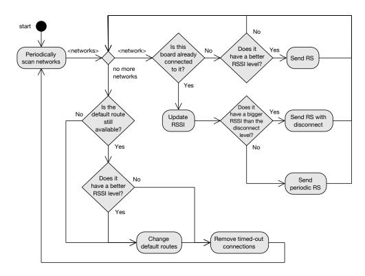
FIGURE 2.17. WAVE networks processing thread in Connection Manager.
