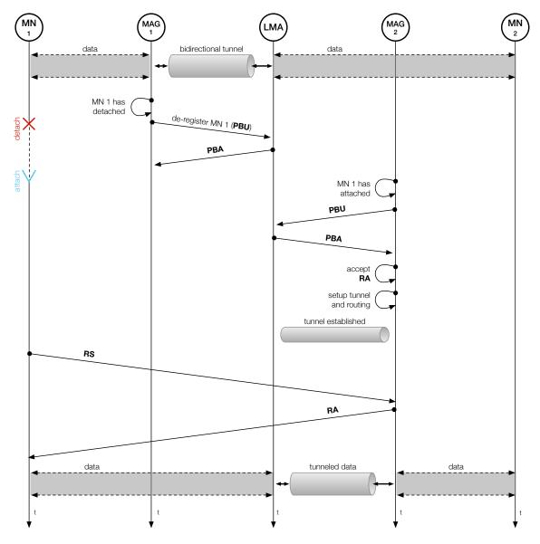
FIGURE 2.7. PMIPv6 message exchange on PoA handover. When a MN transitions from a MAG to another, the respective MAG has the responsibility of checking out the node's disconnection and then send a de-registration message through a PBU message to the LMA, who should respond with a PBA. When a MN re-attaches to a MAG, this should send a PBU to the LMA, waiting for a PBA to set up a tunnel and routing rules. After this, the RS-RA handshake should occur, in order to signal this connection as alive.
