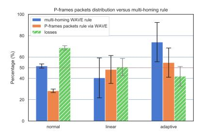
FIGURE 5.7. P-frame packets distribution in comparison with applied multi-homing rule in static 720p experiments. The losses in the plot are a copy of those in figure 5.6.
