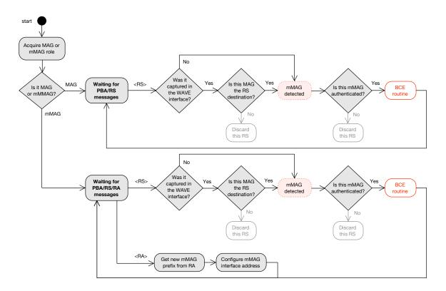
FIGURE 2.11. The MAG and mMAG operation finite state machine.
