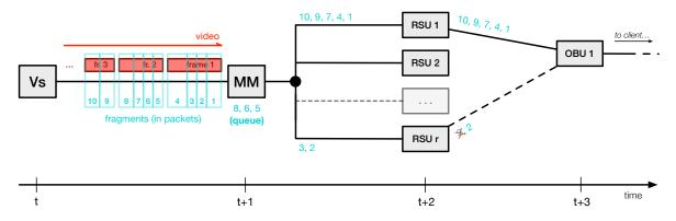
FIGURE 3.2. Load-balanced packet flow, in the mobility manager with a queueing mechanism. While diminishing the queue length at the RSU's interfaces could help parts of frames not to be abundantly lost, and the MM is storing packets until a reliable connection to an RSU appears, this is not a viable solution since it cannot provide us with near-real-time video transmission.
