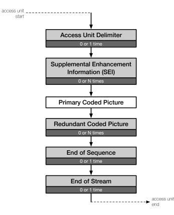
FIGURE 2.21. NAL access unit structure (adapted from [23]).
