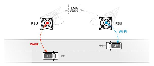
FIGURE 2.9. A simple representation of a VANET in use by two vehicles.
