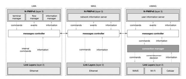
FIGURE 2.14. Integration of a Connection Manager with the background running N-PMIPv6 protocol.
