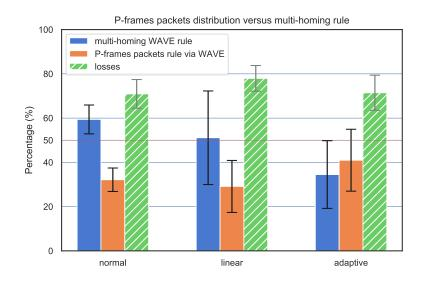
FIGURE 5.9. P-frame packets distribution in comparison with applied multi-homing rule in static 1080p experiments. The losses in the plot are a copy of those in figure 5.8.
