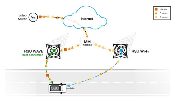
FIGURE 4.1. Using MPEG-4's H.264 standard as video stream input to our system.
