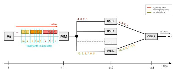
FIGURE 3.4. Load-balanced packet flow, in the mobility manager, considering video segments' context. With this solution, and having in consideration video frames with different priority levels, packets relative to the same segment can be sent through the same RSU. Here, if a set of packets is lost, the video stream can still be visualized, depending on the encoding, which can resolve transmission errors via intra- and inter-frame predictions.
