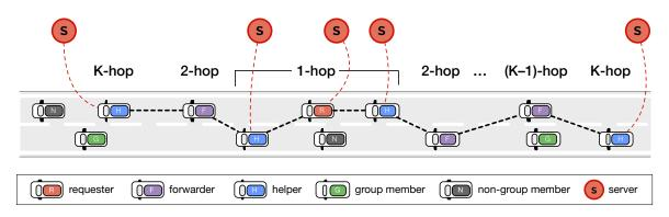
FIGURE 2.23. K-hop CVS scenario proposed by Lee et al (adapted from [37]).
