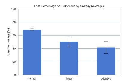
FIGURE 5.6. Loss Percentage on 720p video resolution by strategy in static tests.
