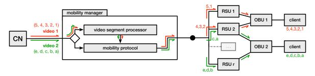
FIGURE 3.6. Multiple video streams under the proposed solution architecture.
