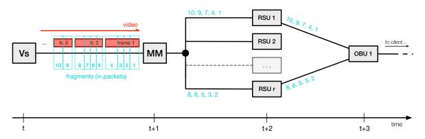
FIGURE 3.1. Load-balanced packet flow, in the mobility manager, per available RSU on the path towards a client. As a video stream enters the MM with frames encapsulated in multiple segments (here represented as fragments), the load-balancing feature will blindly split the flow through its array of available RSUs, disallowing the client to reproduce the video stream, since frames can arrive incomplete to the OBU.
