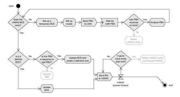
FIGURE 2.12. The MAG and mMAG BCE operation finite state machine.
