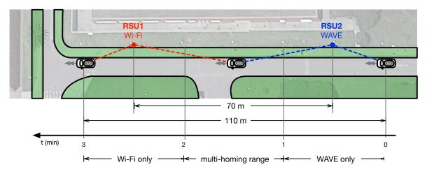
FIGURE 5.17. Representation of the outside tests, on a time axis.
