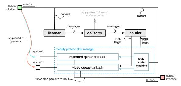
FIGURE 3.9. Global architecture of the proposed system, in detail.
