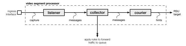
FIGURE 3.7. Architectural components of the video segment processor.
