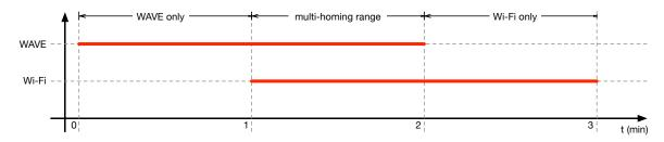
FIGURE 5.11. Representation of the handover tests, on a time axis.
