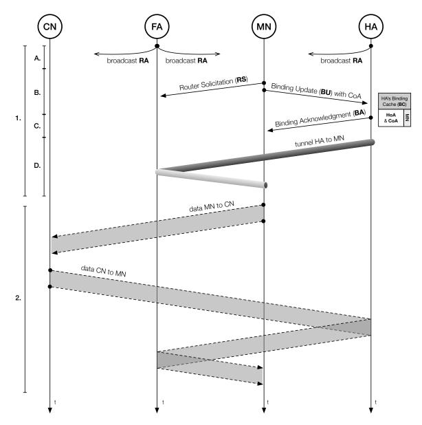
FIGURE 2.5. Messages exchange in MIP. Here are depicted both presentations (1.) and data transmissions (2.) from a MN to a CN, and vice-versa. In the presentation there are four different phases, naming the discovery (A.)—the HA searches for its MNs,— the registration (B.)—the MN registers into its HA or FA,— the binding (C.)—the HA or FA binds the MN's HoA with CoA within a BCE,— and the tunneling (D.)—where a tunnel is created between the HA or the FA and the MN.
