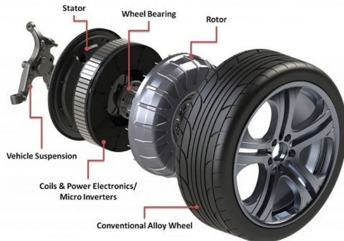
Figure 2.9: Schematic of Protean Electric's in-wheel motor configuration [47].
