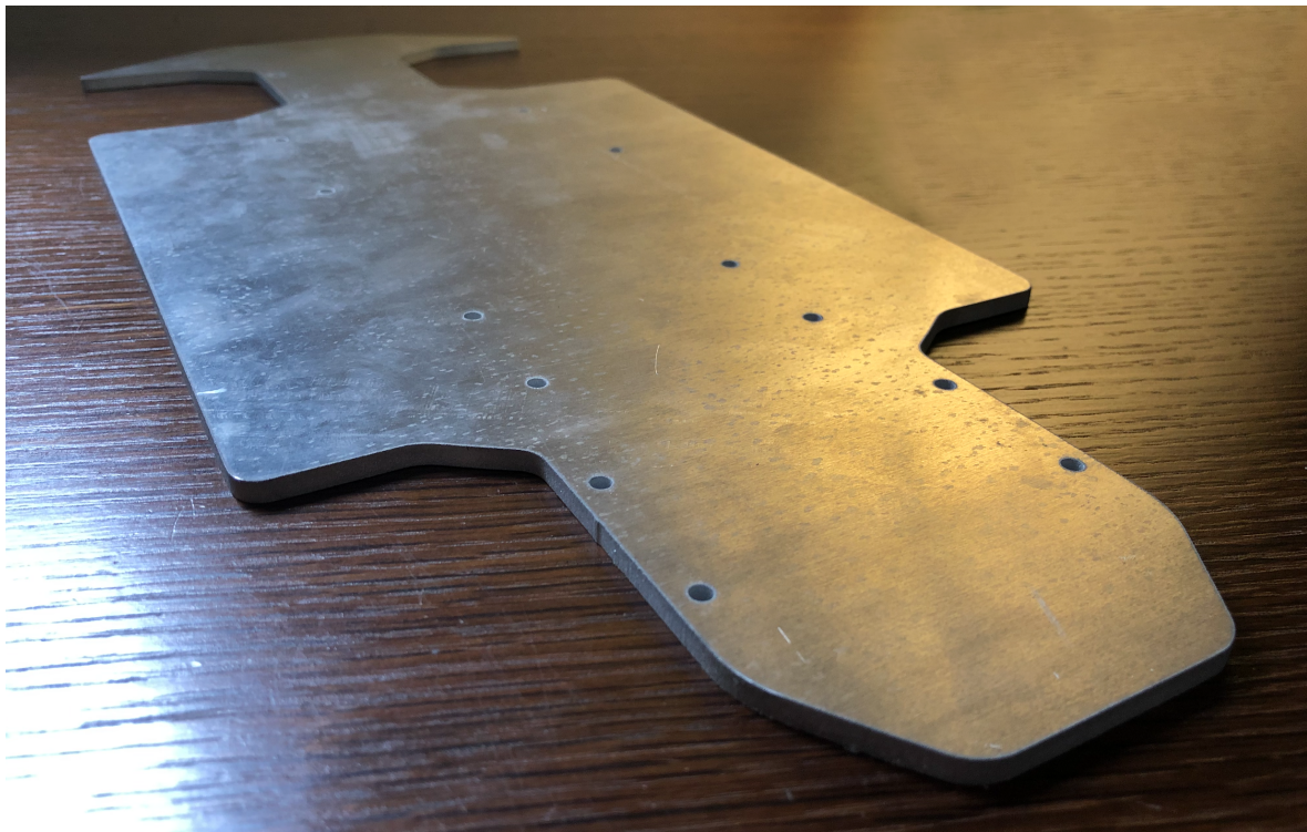
Figure 4.28: Chassis part of the model vehicle before the polish treatment.
