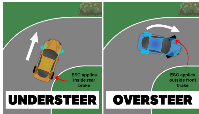
Figure 2.5: Understeer and oversteer situations where ESC is applied, adapted from [29].
