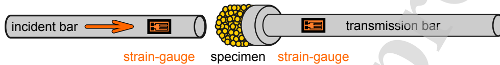
Figure 3: Principle of the direct impact Hopkinson bar methods.
