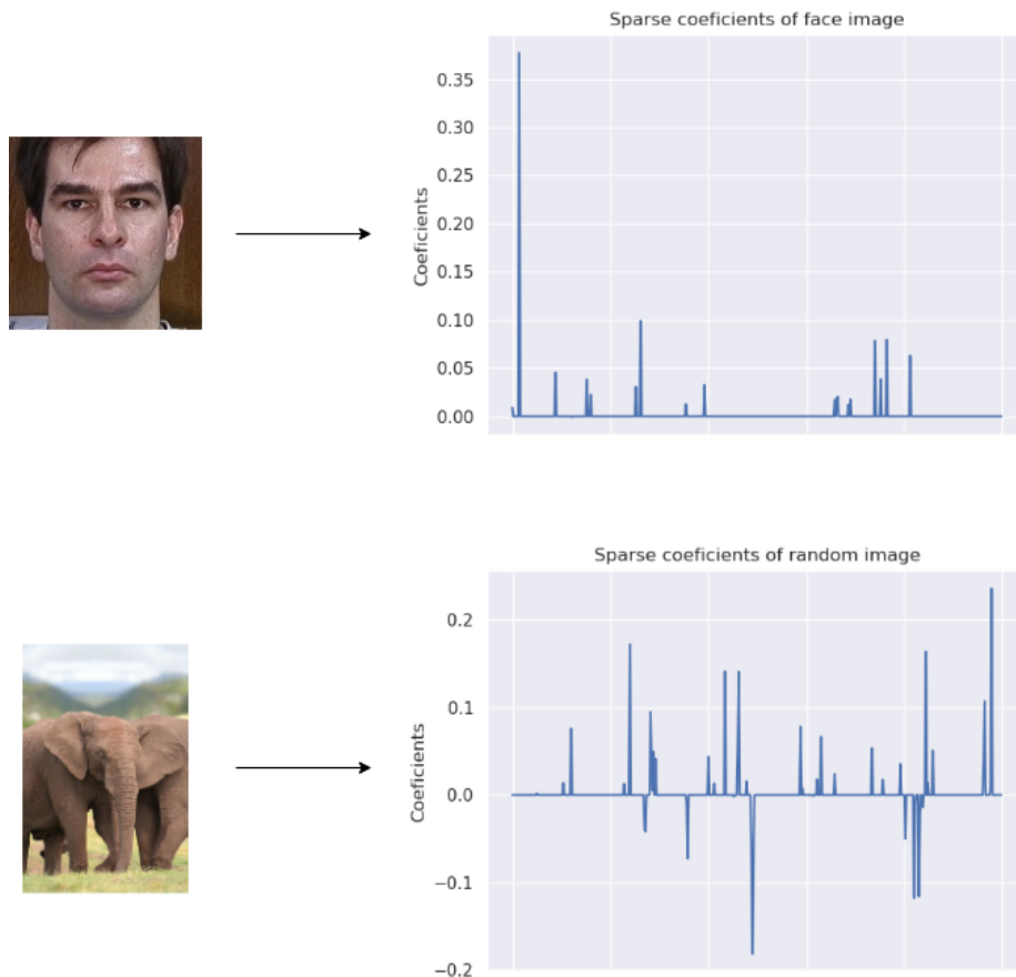
Figure 3.5: Plot of the sparse coefficients \|\mathbf{x}\| of a face image and a random image.
