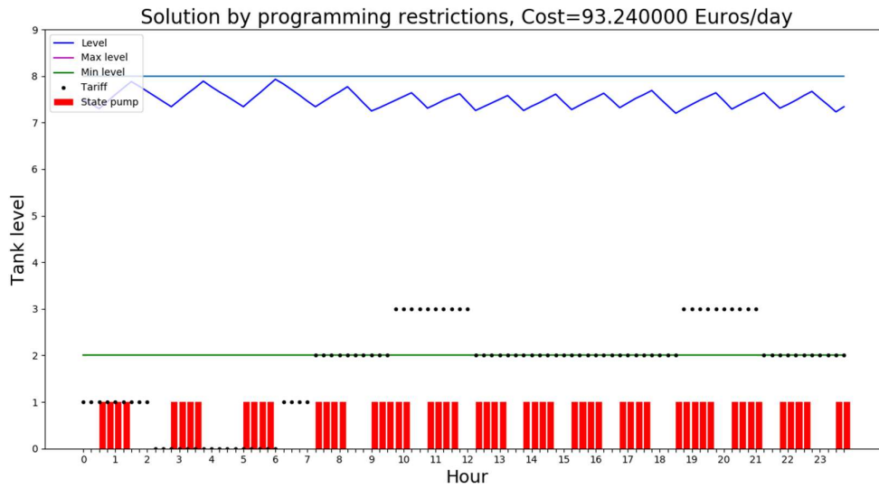
Figure 35. Pumping operation optimized by constraints. Initial level = 7.5m.
