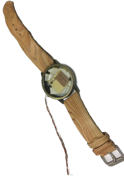
Figure 3.13: Backscatter modulator embedded into the watch.
