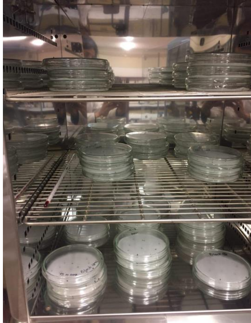
Figure 2.11 The prepared petri dishes with ten seeds of Lepidium sativum and 2mL of extracts of incubated samples (soil and amended soil with 2.5, 5, and 10% 9w/w) (with 3 replicates for each condition), plus five dishes as control (as the replicates).
