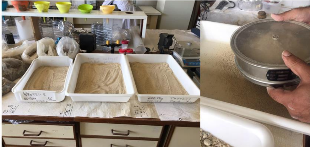
Figure 2. 4 The soil supplied by the pulp and paper industry and collected from its forest soils. The soil was air-dried for three days and then it was sieved through a 2mm sieve.
