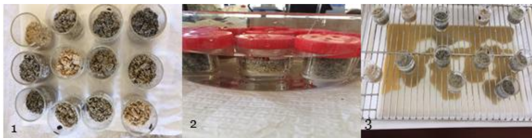
Figure 2. 8 The adopted procedures in order to measure the WHC of the incubated samples, incubated soil, soil amended with biochar (2.5, 5, and 10% w/w), and soil amended with the commercial fertilizer containing mainly \text{CaCO}_3 (2.5, 5, and 10% w/w) (with three replicates for each condition).
