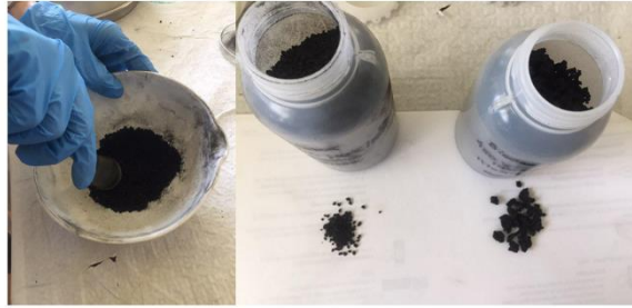
Figure 2. 1 The biochar produced from the sludge of pulp and paper mill effluent at the temperature of 450° C and the rate of 10° C/min. The biochar was smashed and sieved through a 2mm sieve.
