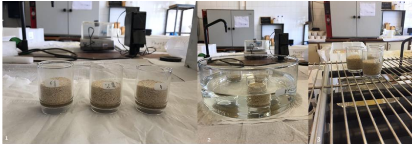
Figure 2. 5 The adopted procedure to measure the WHC of the soil supplied by the pulp and paper industry (with the utilization of 3 replicates).
