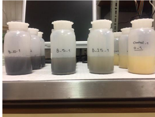
Figure 2. 9 The extracts of incubated samples of soil and amended soil with 2.5, 5, and 10% (w/w) of biochar additive (with 3 replicates for each condition).
