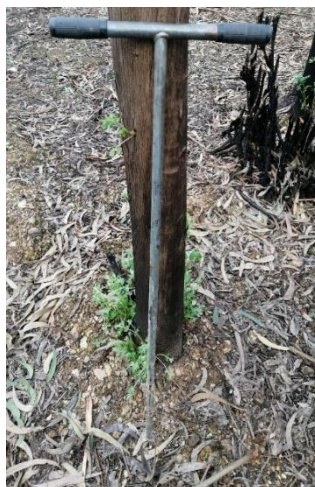
Figure 15 – Auger used for soil collection.
