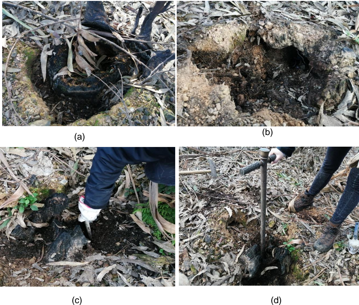
Figure 17- Photos from soil sampling: (a) burnt stump, (b) hole after stump removal, (c) removal of top soil, and (d) Measuring the depth of sampling point.
