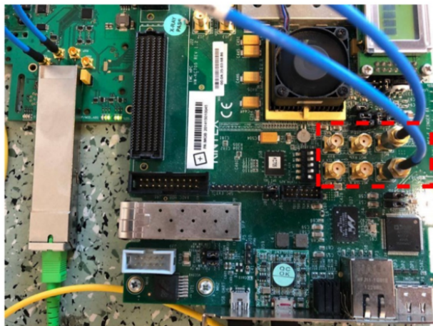
Figure 3.5: GTX SMA Transceiver of Xilinx (KC705 Kintex-7) FPGA [41]
