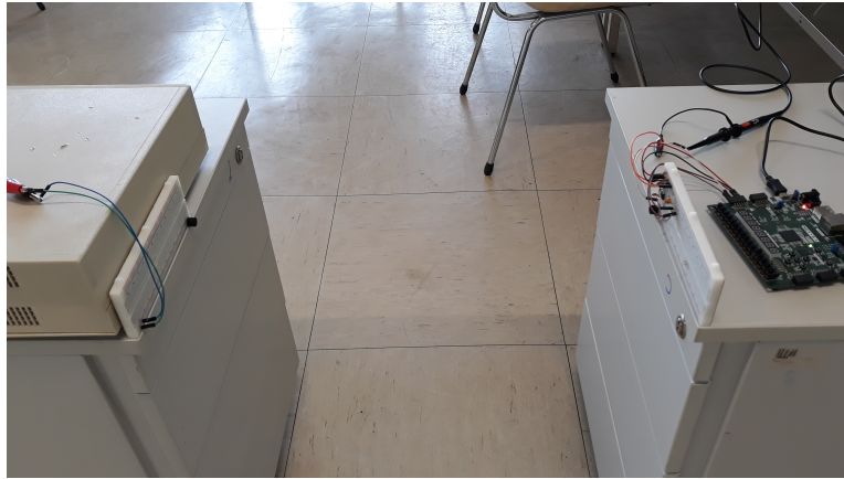
Figure 4.23: Experimental setup for the measurement of the received signal strength as a function of distance; the emitter is on the left side, laying against the function generator, and the receptor is on the right side.
