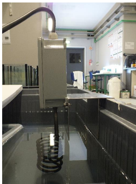
Figure 2.10 – Digitally controlled heater used in CT_{Max} assays.
