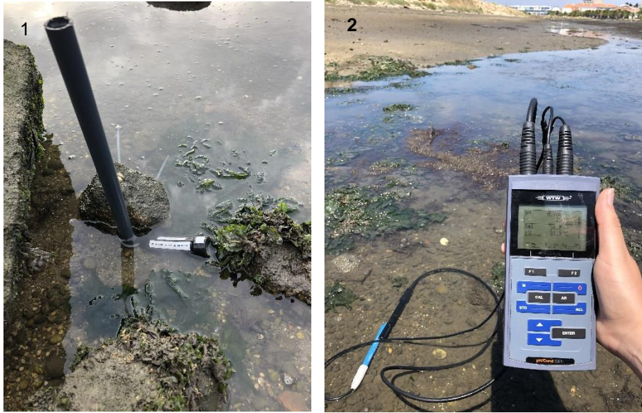
Figure 2.3 – Probes for environmental data: 1) HOBOTemp Pro v2 U22 – 001, Onset, USA 2) conductivity and pH portable meter 3110 SET 1 WTW® (Xylem Analytics, Germany).
