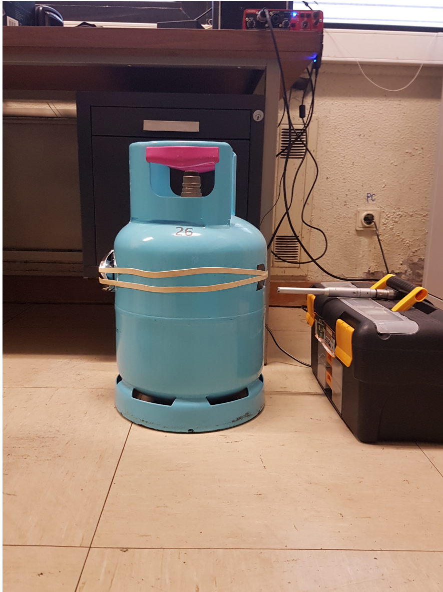
Figure 4.1: Experimental setup with a contact speaker to transmit the chirp signal to the cylinder.
