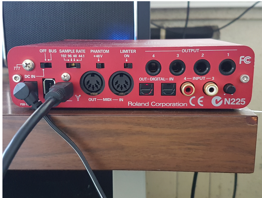
Figure 3.4: Rear connections of the soundboard.
