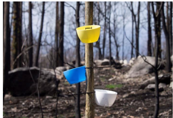
Figure 8 – Aerial pan traps set in a sampling plot.
