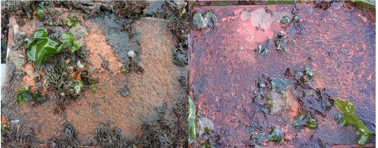
Figure 19: Photographic record of biofouling in blank reference plates showing the presence of ascidians and bryozoans (whitish organisms) and macroalgae (green or brown).
