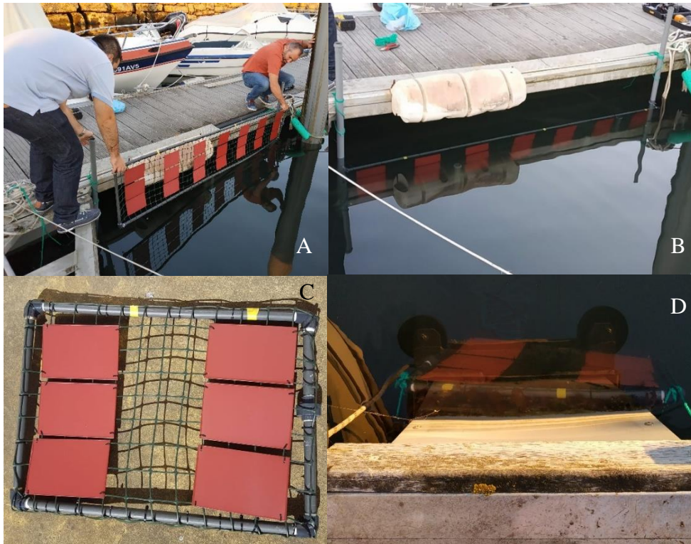
Figure 5: A: Immersion of the system containing 7 out of 9 coatings (Commercial reference, CuPT, CuPT@Zn-Al LDH, Sea-Nine, Sea-Nine@SiNC, SiNC and Cu-Al LDH); B: Immersed Larger system; C: Dry smaller system (with the coatings Zn-Al LDH and Blank reference); D: Immersed smaller system
