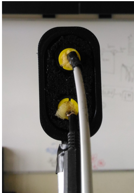
Figure 4.40: Upholstery sponge on the back of the transducers.
