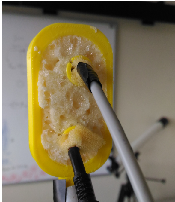
Figure 4.43: Upholstery sponge on the back of the transducers.
