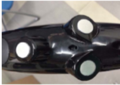
Figure 3.4: Positioning of the ultrasonic sensors. Source:[2]
