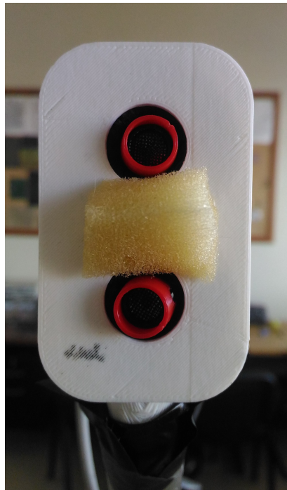
Figure 4.33: 6th version with a piece of upholstery sponge between the two transducers.
