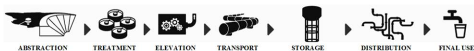
Fig.1 – Main sectors of a water supply system from the source to the end user [9].
