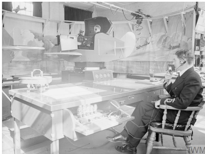
Figure 2.6: Link trainer in use at a British Fleet Air Arm station (Adapted from [20])
