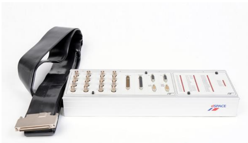
Figure 4.3: CLP1104 Connector and LED Panel (Adapted from [64]).
