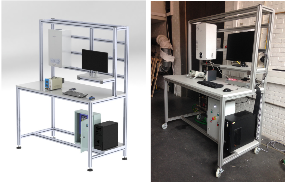
Figure 3.2: Comparison between the 3D model and the real virtual test bench.
