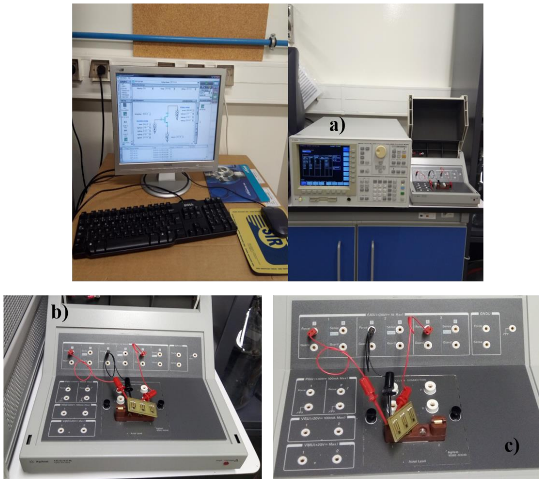
Figure 4 - Apparatuses for the acquisitions of electrical measurements: a) semiconductor parameter analyzer; b) open test fixture with a printed circuit board fixed and drain (D), gate (G) and source (S) of the FET is linked to the respective terminals; c) zoom image of the connection of the FET electrode to the test fixture.
