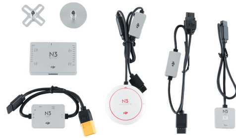
Figure 2.2: DJI N3 flight controller with included power management unit and GPS sensor. [29]
