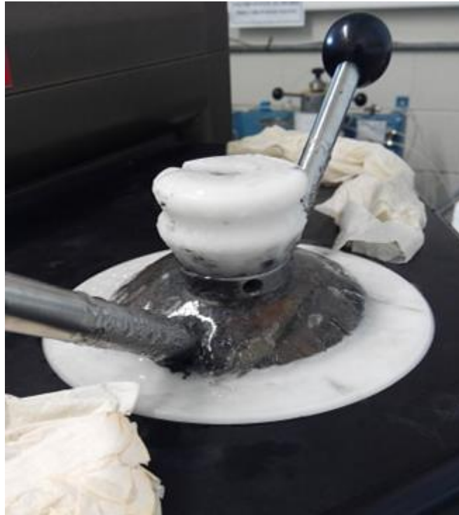
Figure B1 – Frozen pressure vessel top during the assay at 25 MPa/-5 °C.
