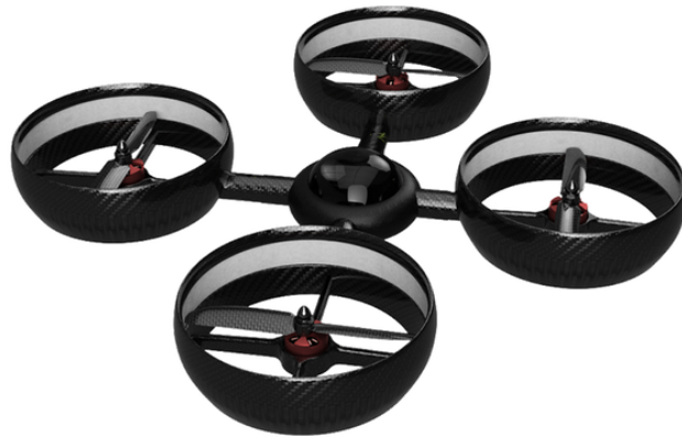
Figure 2.8: Dotterel drone: lightweight propeller shrouds comprising sound-absorbing acoustic materials [24].
