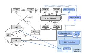
Figure 3: Proposed mobile network architecture.
