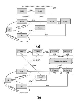
**Figure 1:** 3GPP and non-3GPP network integration in a: (a) current EPC architecture. (b) SDN/NFV EPC architecture.
