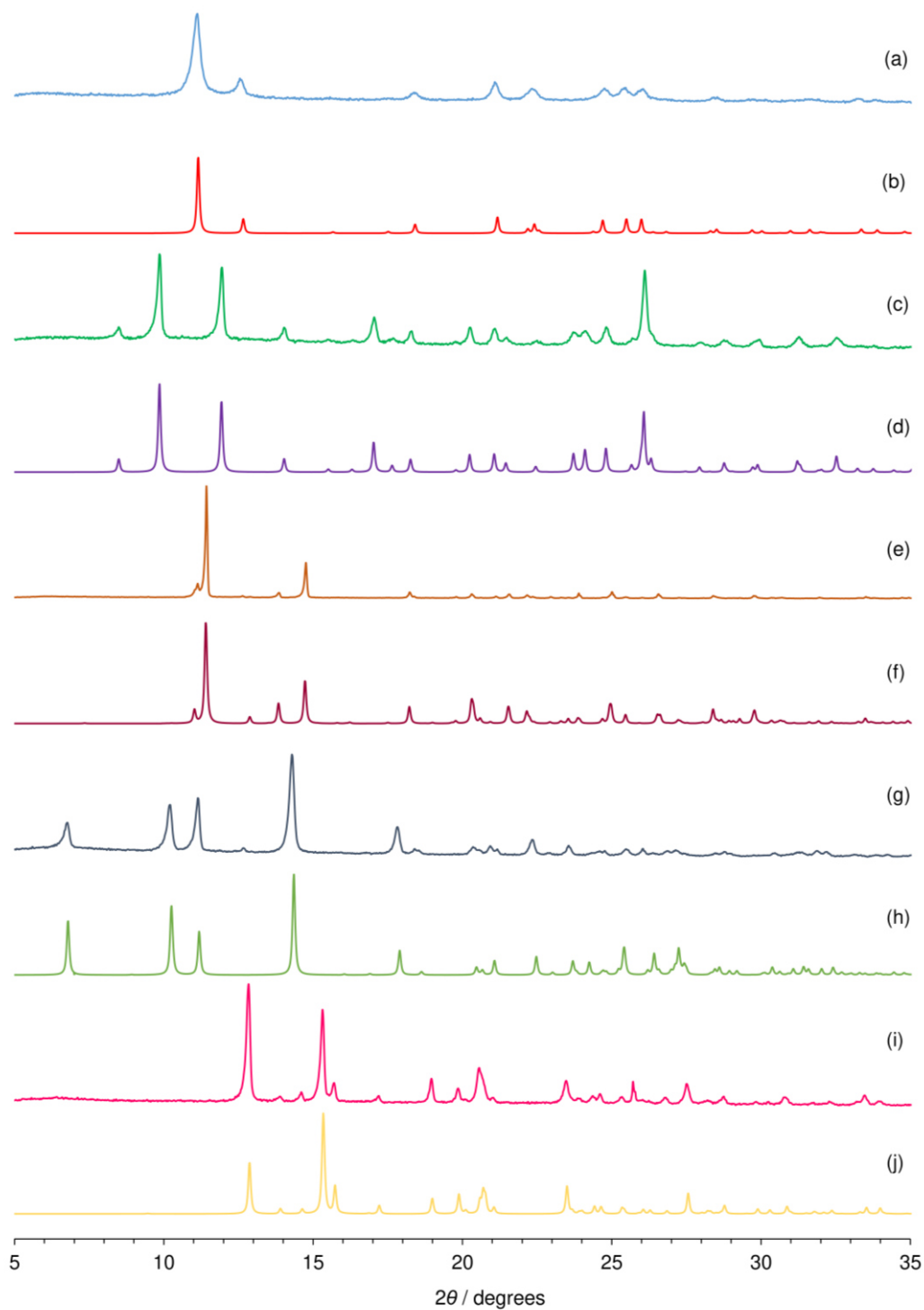
Figure 6.3. Experimental (a, c, e, g, i) and computed (b, d, f 44,5 h 7,8 , j 9 ) PXRD patterns of (a, b) 1 , (c, d) 2 , (e, f) 3 , (g, h) 4 , (i, j) 5 .
