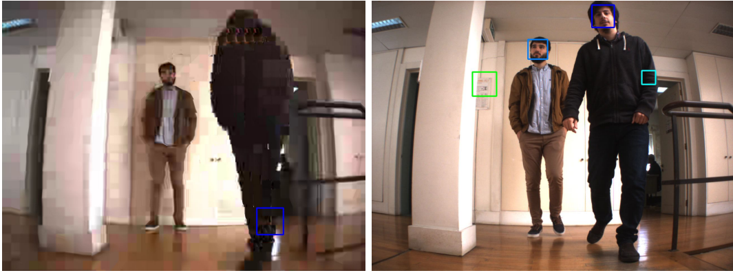
(a) Image compressed with H.265 and CRF 51. (b) Image compressed with Theora quality level 10.
