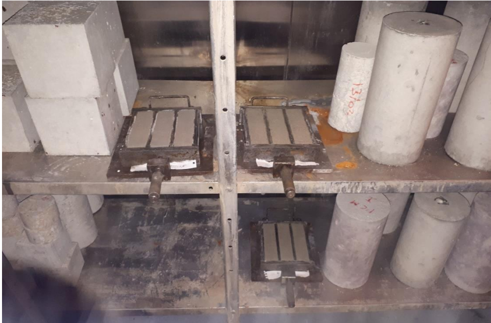
Figure 3.3.3-1: Mixtures DDL-H 2 O (top left), DDL-NaOH (top right) and DDL-KOH (bottom) from Trial one undergoing curing in a climate chamber at 95% relative humidity.
