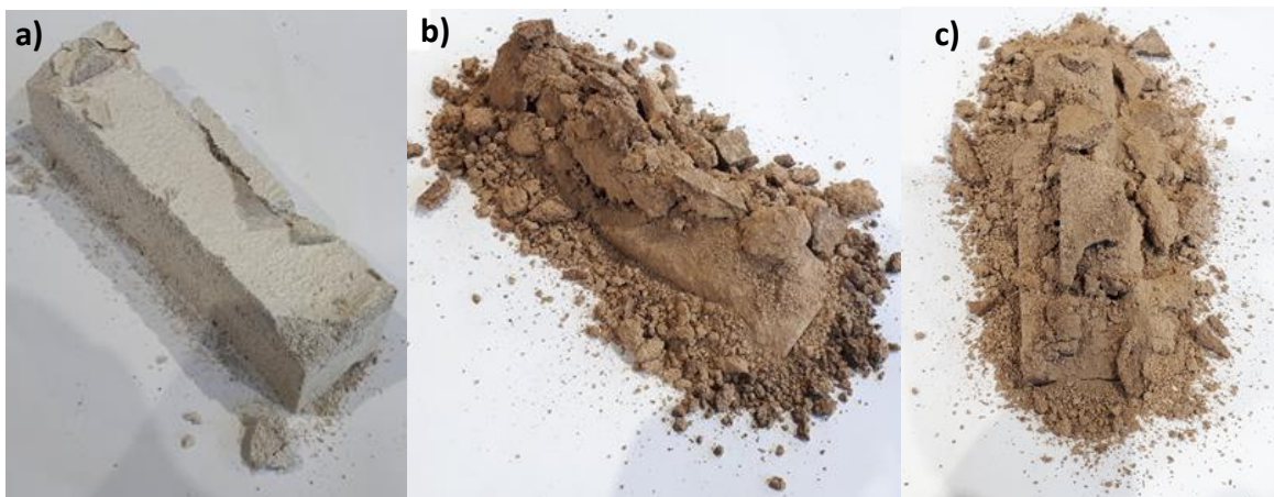
Figure 4.1.4-2: Results of the Trial four experimental procedure. a) DDL-H 2 O. b) DDL-NaOH. c) DDL-KOH.
