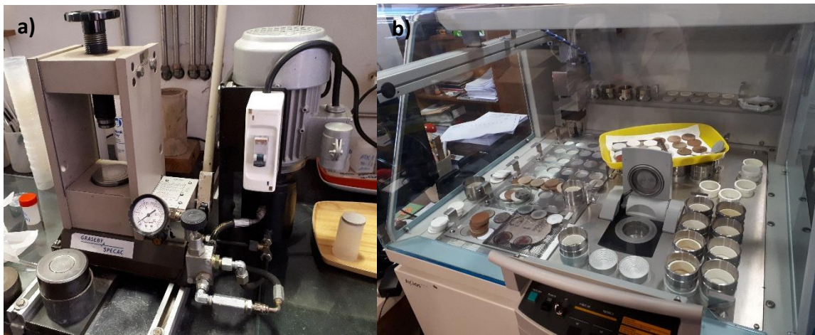
Figure 3.4.1-1: a) Hidraulic press used to create sample disks. b) X-Ray Fluorescence analyzer with several sample disks visible.
