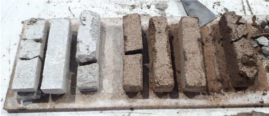
Figure 4.1.3-1: Results of Trial three experimental procedure; three DDL-H 2 O specimens, three DDL-NaOH specimens and one DDL-KOH specimen, respectively, from left to right.
