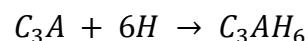
Equation 2.1.1-2: Chemical equations for the hydration of Alite, Belite and Celite respectively in Cement Chemist Notation (CCN).
