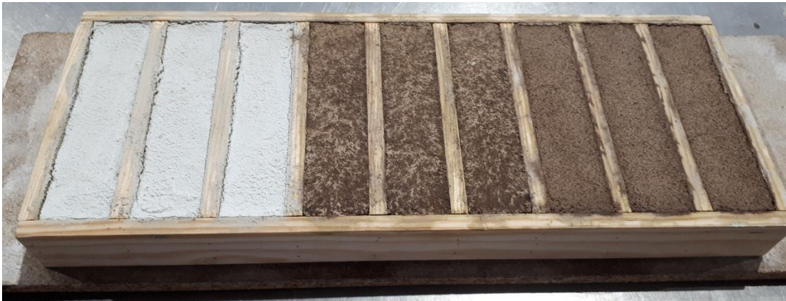
Figure 4.1.4-1: Trial four specimens after the curing period; three DDL-H 2 O specimens, three DDL-NaOH specimens and three DDL-KOH specimens, respectively, from left to right
