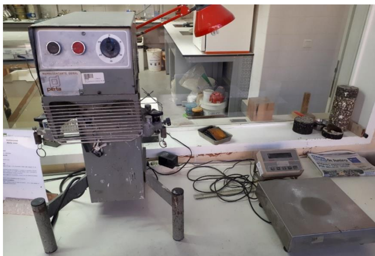
Figure 3.3.2-1: Mortar mixer (left) and digital scale (right) used in the mixing procedure.
