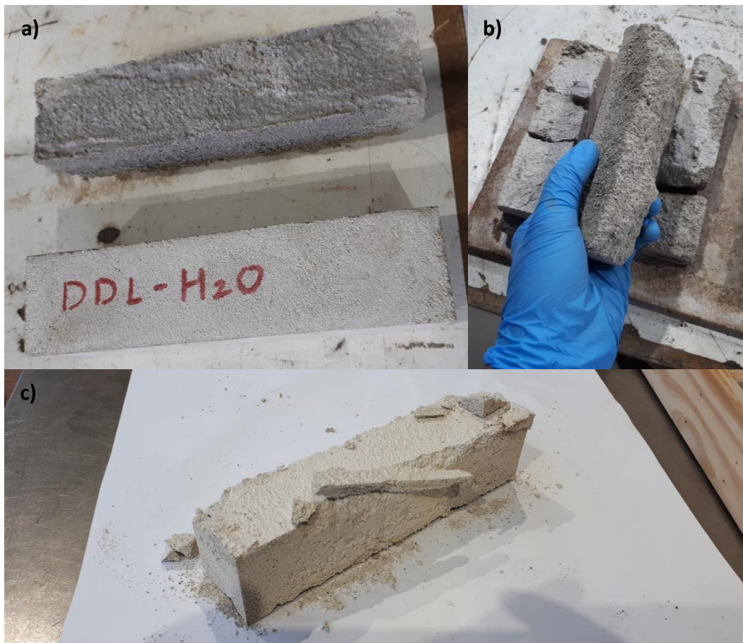
Figure 4.2.1-1: a) comparison between Trial one (below) and Trial three (above) DDL-H 2 O specimens. b) Trial three DDL-H 2 O specimens. c) close up of Trial four DDL-H 2 O specimen.
