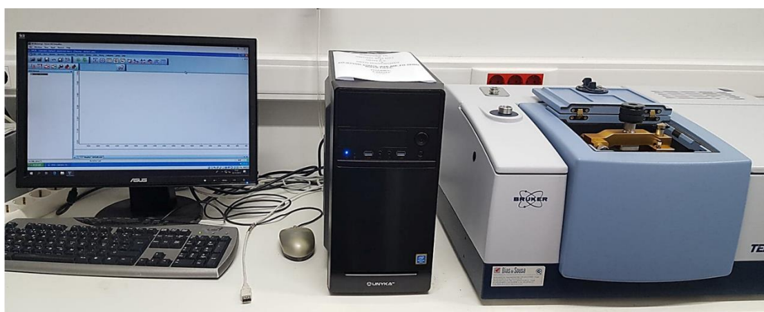
Spectrum ← FFT (computer) ← Interferogram ← Spectrometer (source, interferometer, sample and detector)
