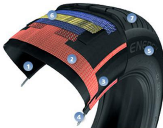
Figure 1.1 – Tire cross section, according to Michelin [1]. The tire is divided in 7 different critical parts: the inner liner (1), the casing (2), the apex (3), the bead (4), the sidewalls (5), the belts (6) and the tread (7).
