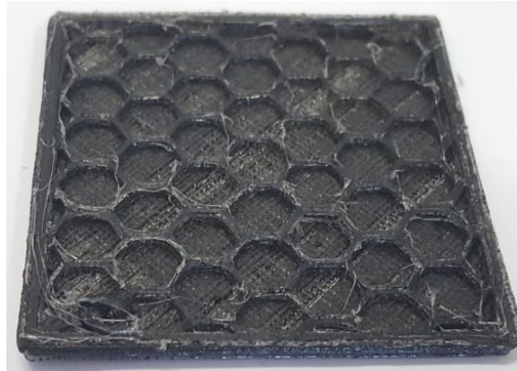
Figure 3.13 – First printing attempt of an “egg box type” panel designed with a quadrangular base of 5 cm side, with four quadrangular pyramids of 1 cm of height. Panel printed with filament F2, with a 0.6 mm nozzle diameter and an extrusion temperature of T = 170^{\circ}\text{C} .
