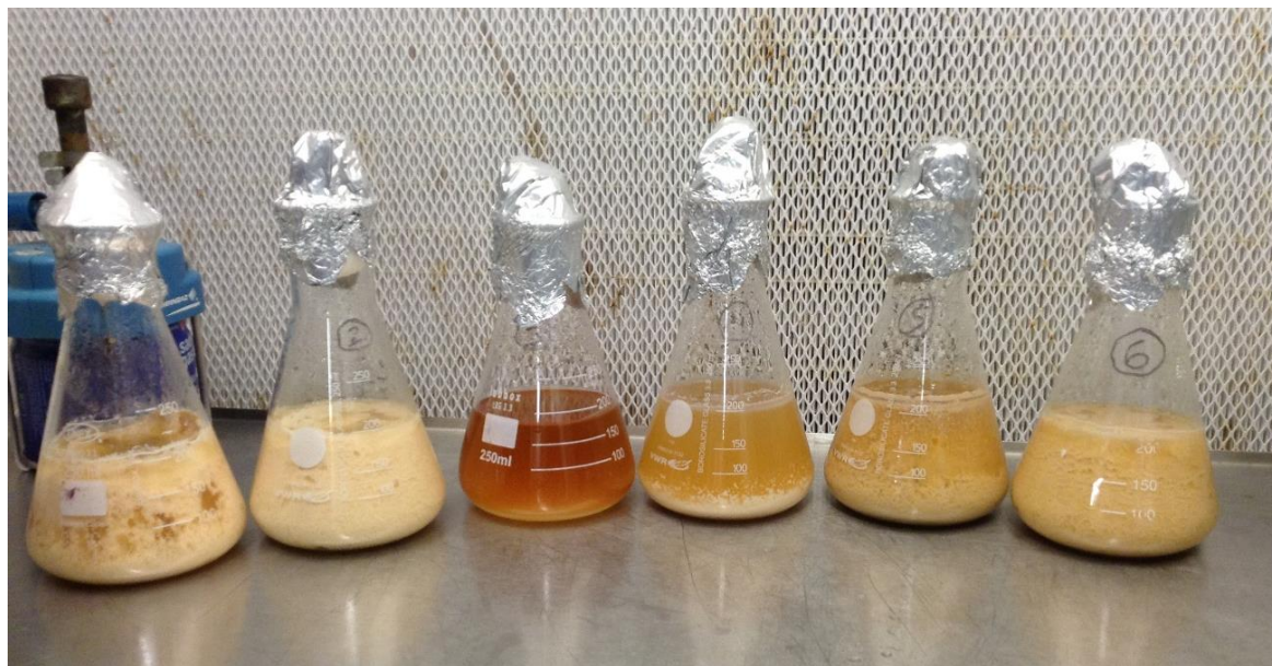
Figure 17. Physical appearance of cheese whey samples, after autoclaving, with the precipitated protein aggregates. From left to right: CW1, CW2, CW3, CW4, CW5, CW6.
