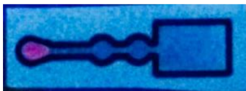
Figure 34: Application of \text{EuW}_{10}@SiO_2\text{-DNA} nanoparticles on a \mu\text{PAD}
