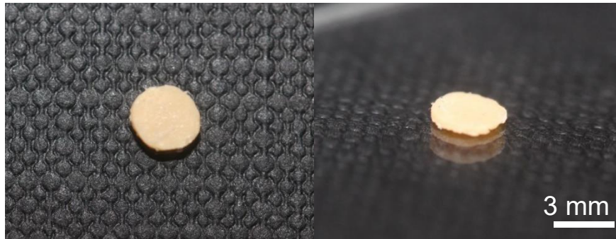
Figure 13. Micrographs of colloidal gel moulded to a disk shape by using a 3.5 mm PDMS mold.
