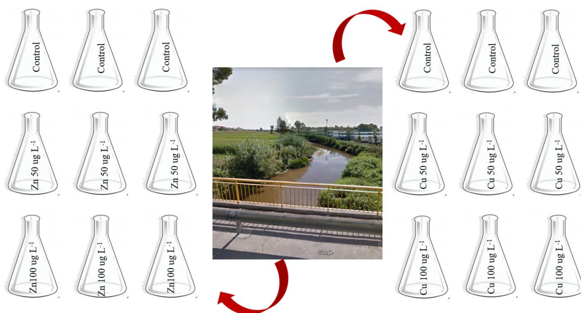
Figure 6: Microcosm experiment setup, 3 L of water (150 mL for each erlenmeyer) was collected at April 11, 2018 for copper assay; and at June 22, 2018 for zinc experiment;
