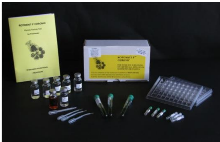
Figure 20. Rotoxkit F (MicrioBioTests, Gent, Belgium) hatching kit. (Source: http://ambifirst.pt/produtos/microbiotests-toxkit/ )
