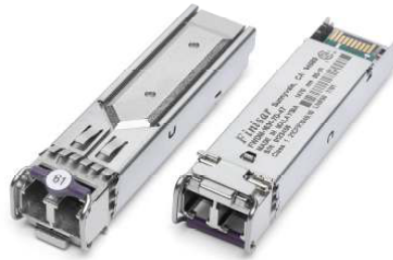
Figure 4.6: Small Form-factor Pluggable (SFP) transceiver (retrieved from [Fin09b]).
