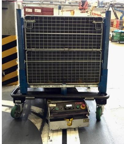
**Figura 18** - AGV (Automated Guided Vehicle).
