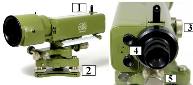
Figure 3. 8 - Theodolite Wild-N3 (Zapata, 2017).
