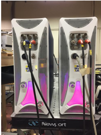
Figure 3. 19 - Two power supply for the blue laser system type BSL200 CFR300 (Antal and Tagadó, 2010).
