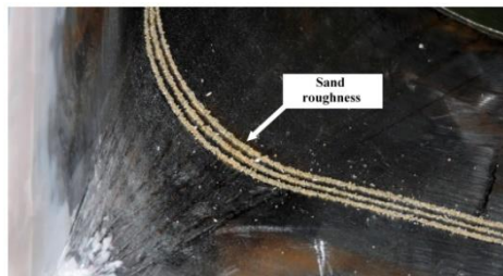
Figure 3. 2 - Picture of the sand roughness on the entrance of the WAABLIEF (Zapata, 2017).
