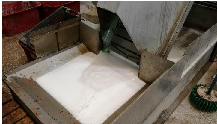
Figure 38 - Cooling conveyor entrance
