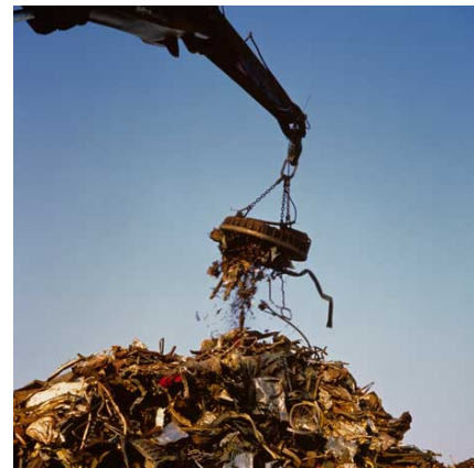
Figure 2.5: Example of an electromagnetic gripper used to lift ferromagnetic objects.
