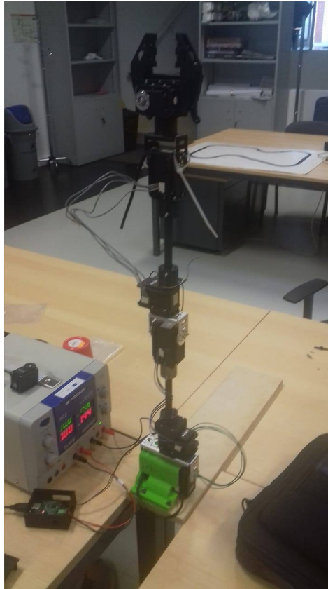
Figure 3.22: Anthropomorphic arm mounted vertically on plywood.
