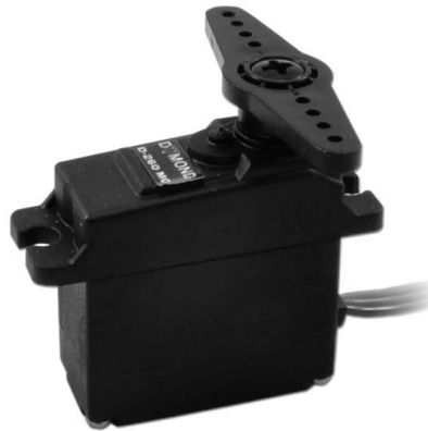
Figure 3.12: Example of a hobby servo.
