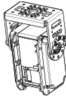
Figure 3.3: Representation of the servo as a pitch movement.
