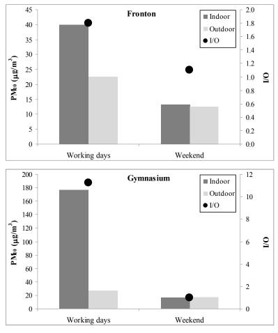
Fig. 2. PM<sub>10</sub> concentrations and indoor/outdoor ratios.
