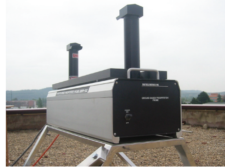
FIGURE 1: Ground-Based Precipitation Probe (PMI Model GBPP-100) installed at the University of León.
