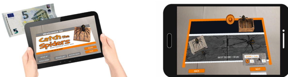
Figure 4 – Veracity augmented Reality: A) Mobile Device running the main game, the device camera recognizes the marker and deploys the VR in top of it, in the respective device screen; B) Developed Virtual environment [16]
